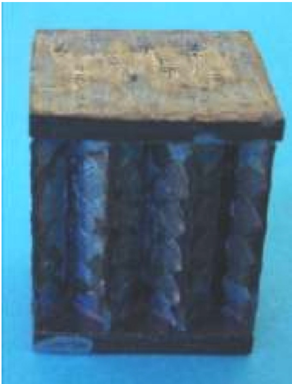
Fig. 6. Sandwich panel brazed by one foil of TiCuNi.
