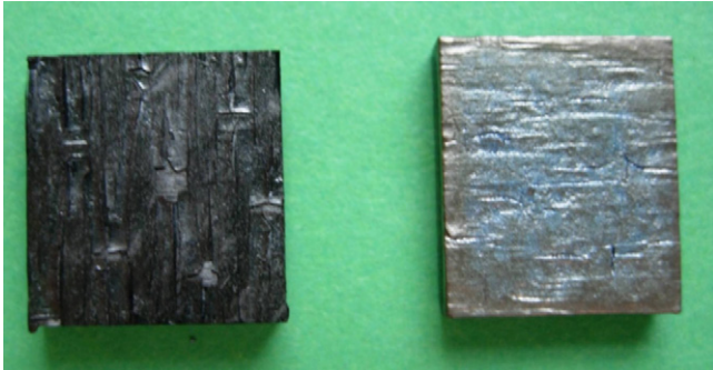
Fig. 2. Macrographs of as-received C/C skins before (on the left) and after (on the right) the wettability tests by TiCuNi.
